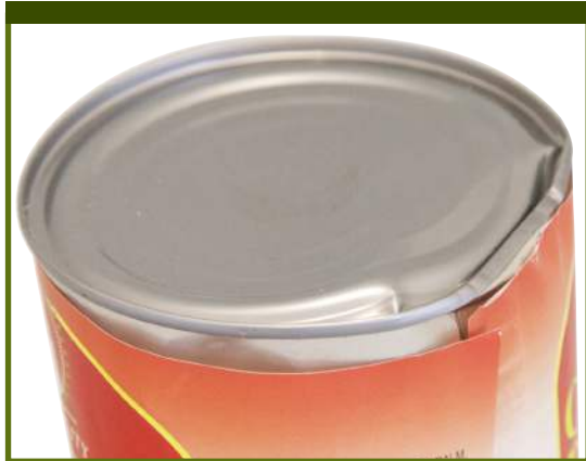
Severe dent in seam
